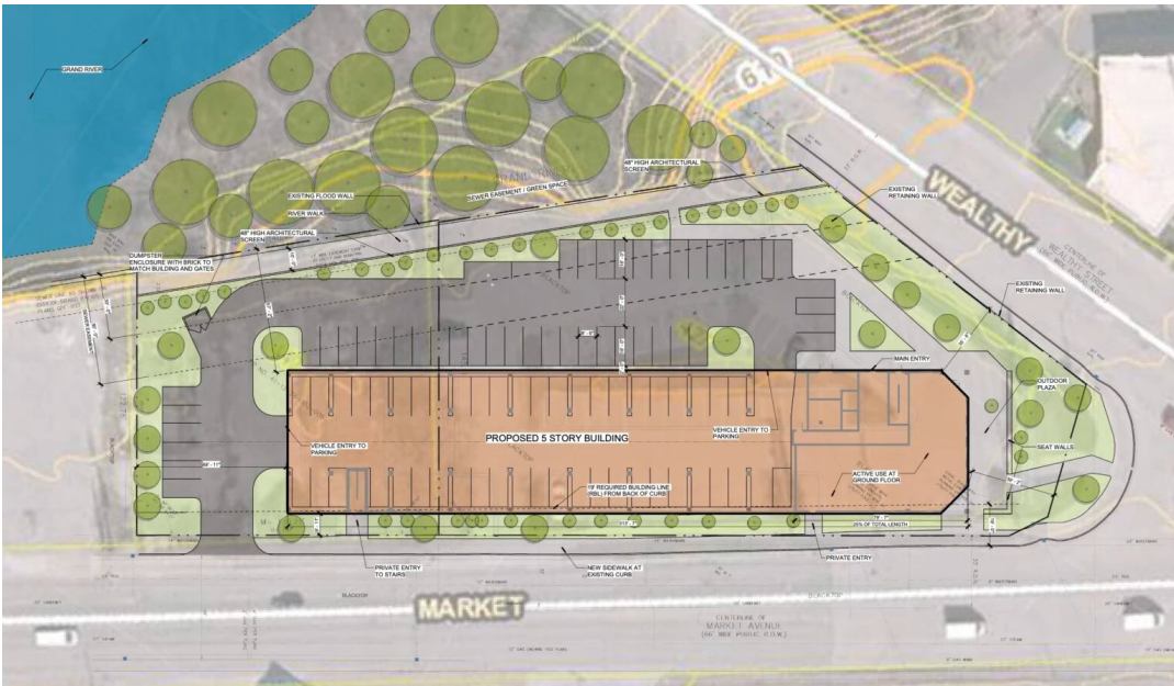
A site plan for the proposed project at 427 Market show surface parking located between the building and the river. Credit: Hooker DeJong Inc.
